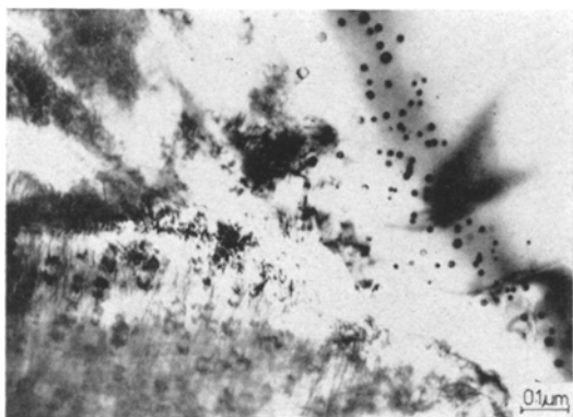
Figure 3 Sub-micron \delta particles in martensite and also present in the \alpha -phase close to the \alpha /martensite interface.
